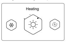
Press ( or ) to change the operation mode. Three modes are optional:, Heating, Cooling, and Auto.
